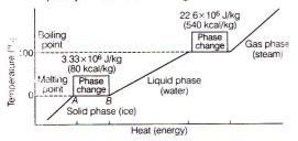
For 1 kg mass  $H_B - H_A =$  Latent heat of fusion.
